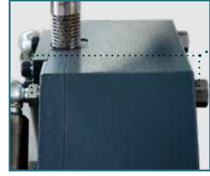
Yan Dayama Ayarı Adjustable guide rolls
