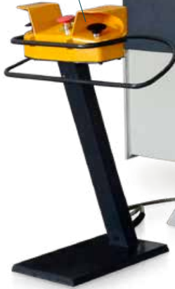
Çift El Kontrol Paneli Two Hand Control
